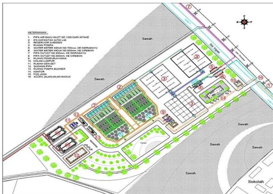
Picture 1 – Layout of Jatigede Water Supply System
